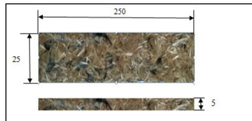
Fig. 3.2 Tensile test specimen
