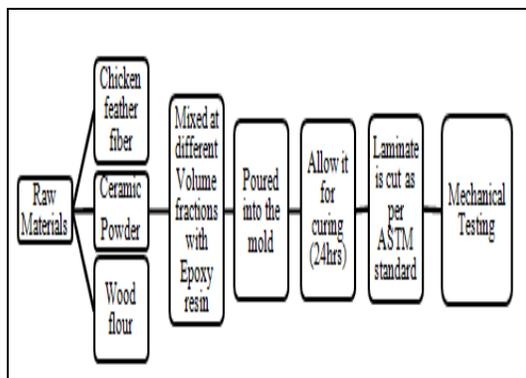
Fig 2.4 Hand Layup Process flow chart
