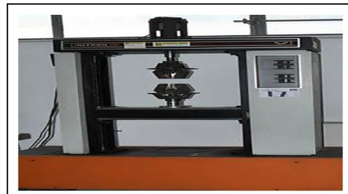
Fig. 3.1 UTM setup for Tensile test
